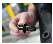
5.) Install couplers and clamps to intake tube as shown.
