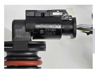
With the plastic removed, the connector should seat to the sensor and appear as shown.
