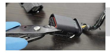
Use a small pair of wire snips, or a Dremel tool & cut-off wheel to remove part of the plastic from the engine harness cam position sensor pigtail.
