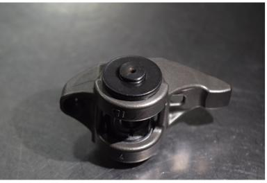
STEP 16: SLIDE THE RETAINING WASHER OVER THE TRUNNION BODY.
