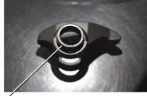
STEP 5: PLACE ONE ROLLER BEARING (PART ID #2) ON TOP OF THE ROCKER WITH THE WRITING SIDE FACING \_ OUTWARD. CENTER THE BEARING WITHIN THE ROCKER ARM OPENING.
