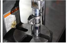
STEP 3: GENTLY PRESS THE 13MM SOCKET INTO THE OEM ROCKER. EFFECTIVELY PUSHING OUT THE OEM BEARING. IMAGE ABOVE SHOWS THE 13MM PRESSED INTO THE ROCKER AS DESCRIBED.
