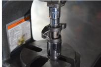
PLACE THE ROCKER FLAT SIDE DOWN CENTERING THE OEM BEARING INSIDE THE OPENING OF THE 22MM SOCKET. PLACE THE 13MM SOCKET ON THE CENTER OF THE BEARING FROM ABOVE SANDWICHING THEM BETWEEN YOUR PRESS
