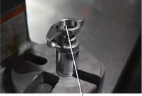
STEP 4: RELEASE THE PRESS AND RÉMOVE THE 13MM SOCKET. YOU'LL SEE THE OEM BEARING HAS BEEN SUCCESFULLY PRESSED FREE FROM THE ROCKER.
